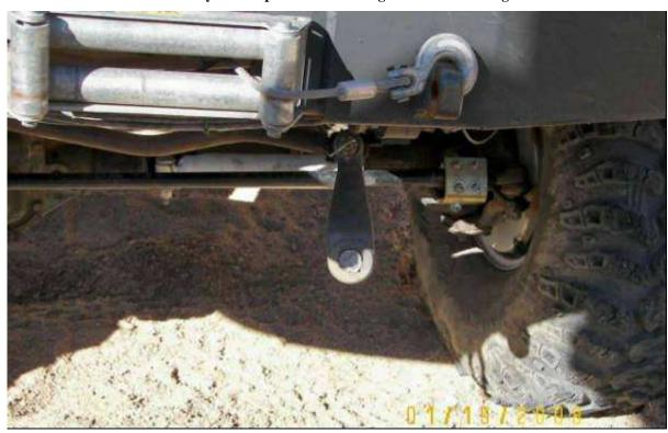
The hanging down thing shouldn't be hanging down. Classic steering gearbox sector shaft sheer caused by tires twice the weight and 33% taller then the factory thought would be put on there.
