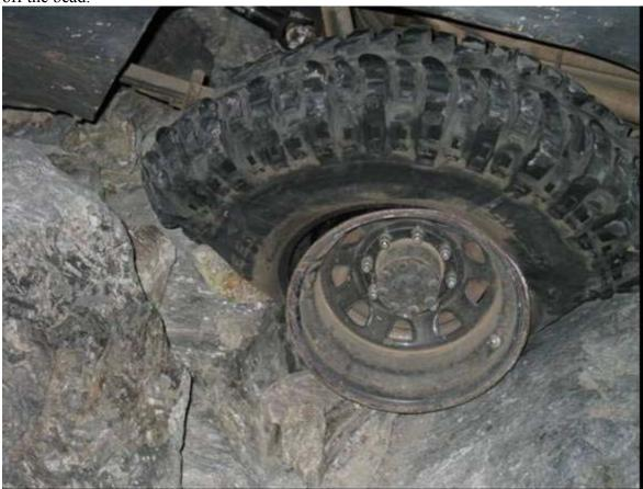
Believe it or not I drove the K5 back 8' on this tire and then we reseated it without removing it from the axle.
