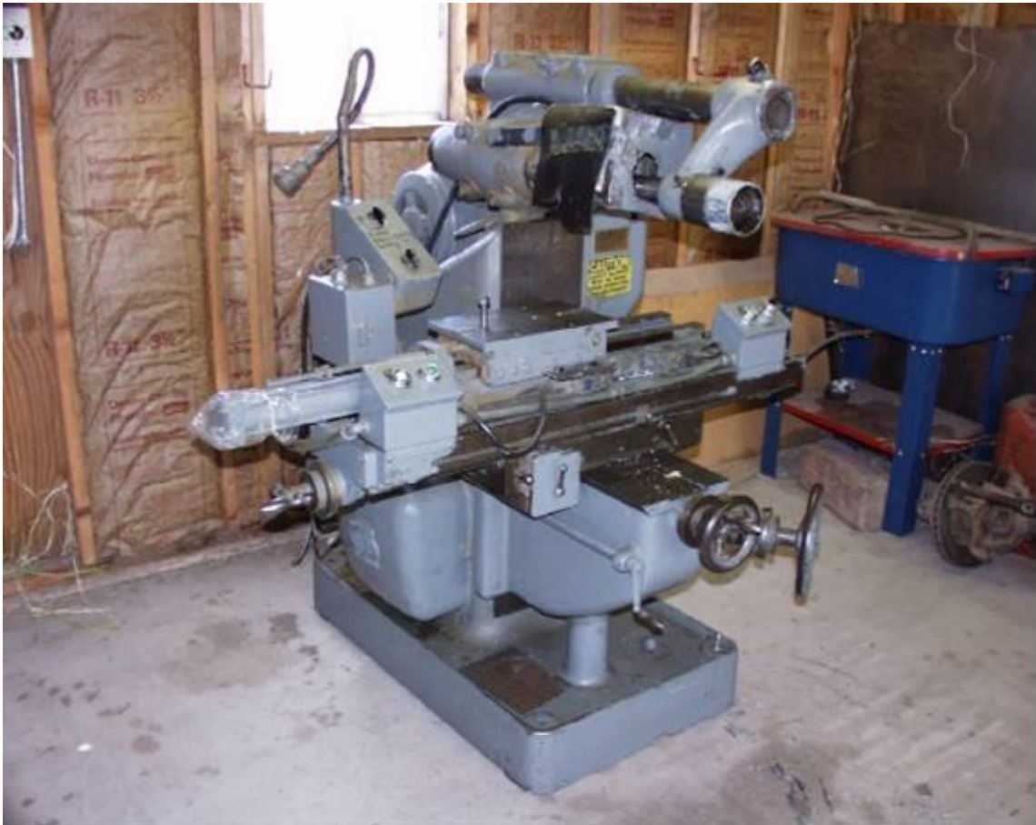
The latest addition to the Graham family, it's a 5hp horizontal/vertical mill.
