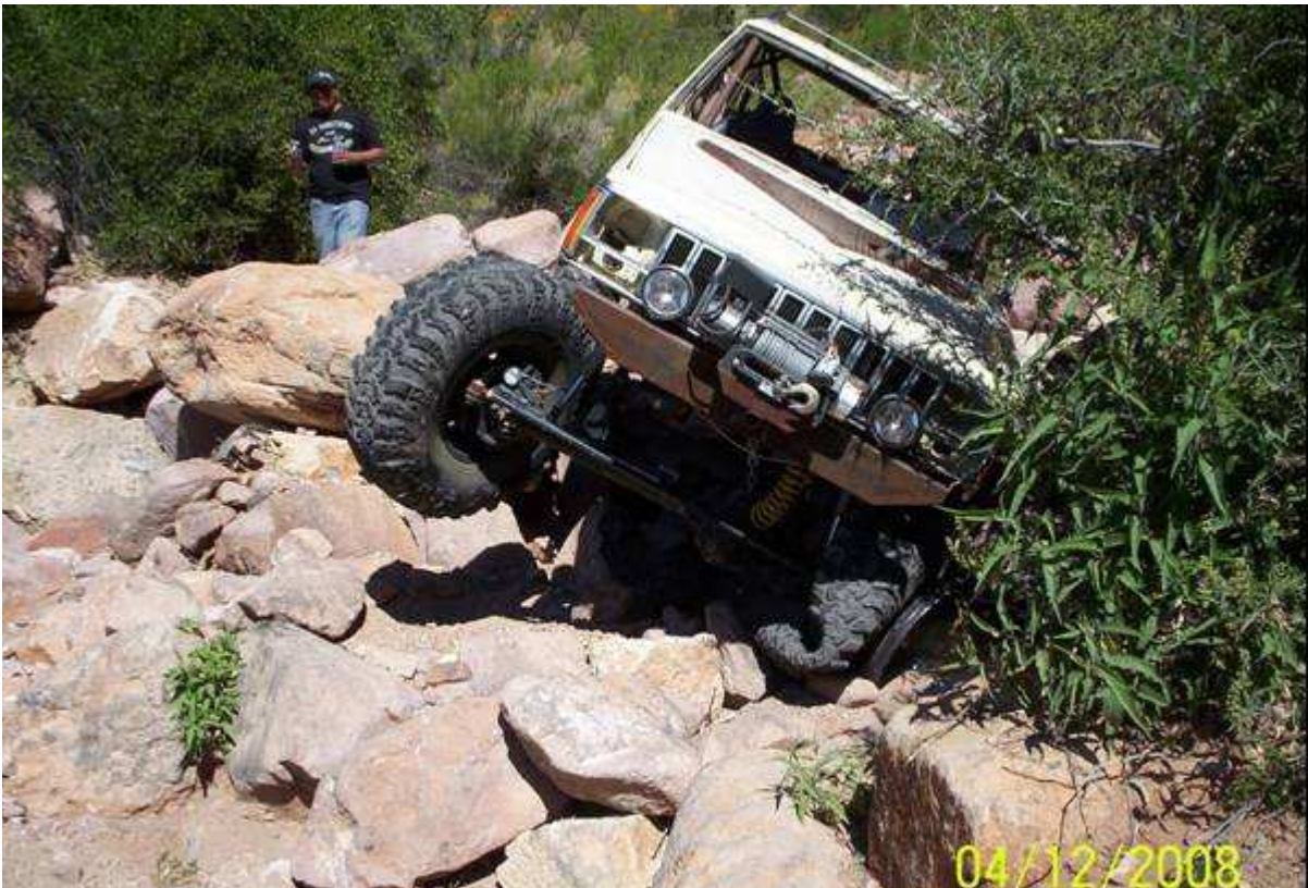
Low tire pressure on a light rig equals debedded tire.
