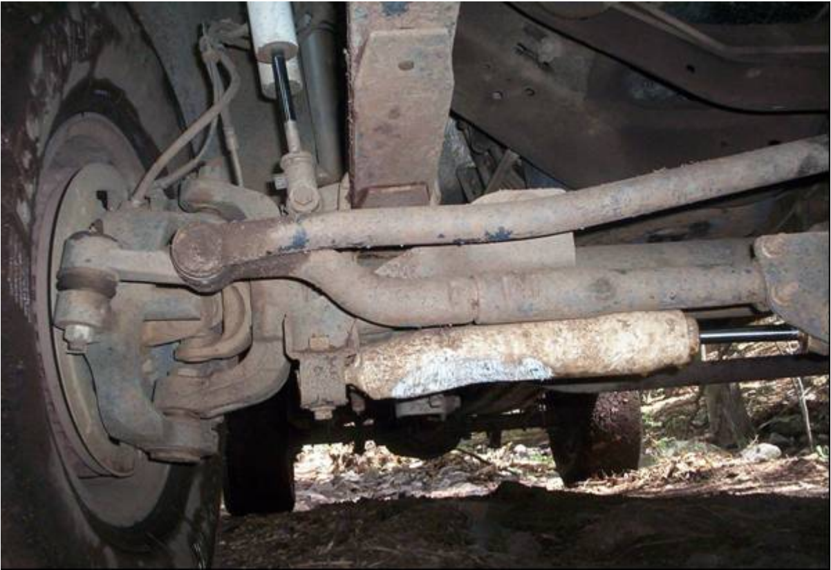
Funny place to put a steering dampener, it had to be removed to continue on the trail.
